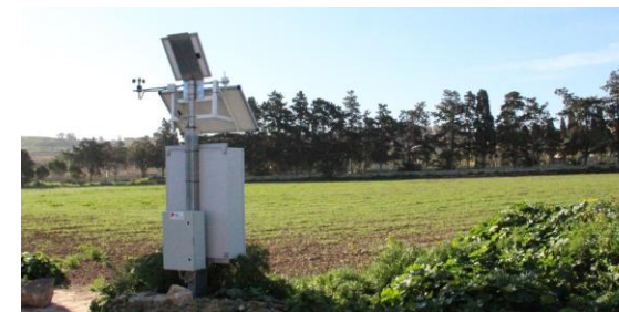
Commissioned monitoring station (Ghammieri) – Forming part of the unsaturated zone monitoring network
