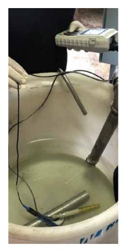
Figure 5. Measuring the conductivity of the permeate
