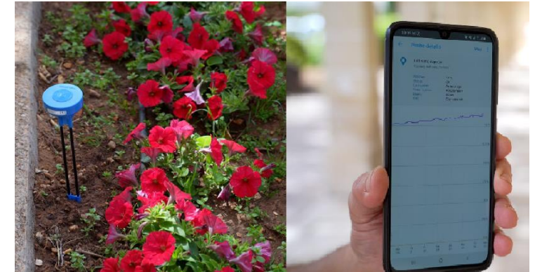
Activity 7 - Soil moisture sensor and mobile app integrated for efficient irrigation.
